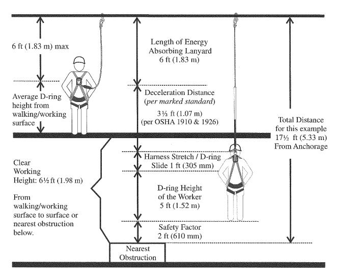
⚠ Caution: If an energy absorbing lanyard is used in conjunction with a cross-arm anchorage connector, other anchorage extension, vertical lifeline, or horizontal lifeline, the additional length of the anchorage connector, or sag from the lifeline must be taken into consideration during the clearance calculation process.
